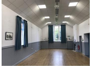
Last year we replaced the convector heaters fitted about 20 years ago with infra-red heating and a dropped ceiling incorporating LED lighting. We insulated the space between the ceiling and roof, saving 50% of electricity usage and giving a comfortable temperature even in the coldest weather and improved acoustics.
